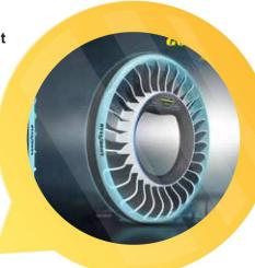
collaboration between NASA and 800 load-bearing springs, which provide stiffness and flexibility, as well as puncture-proof toughness.
